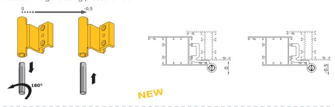
Adjustable bottom hinge: lateral +/- 1 mm (can be carried out with the leaf assembled)
