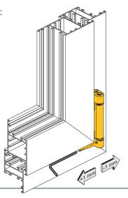
Adjustable bottom hinge: vertical -1 / +2 mm (can be carried out with the leaf assembled)
